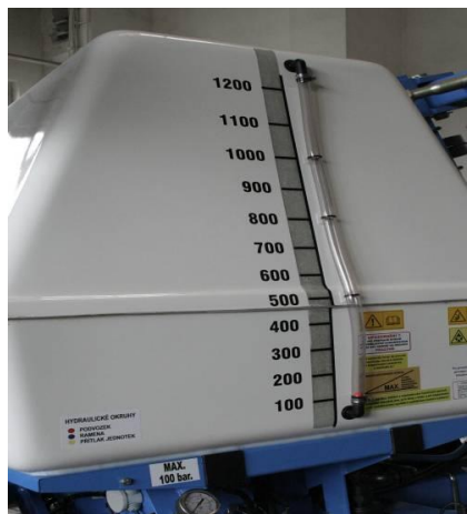
Fig. 1 Fertilizer Tank with Level Gauge
