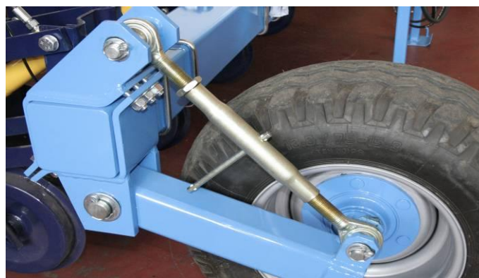
Fig.11 Adjusting Screw of the Front Travelling Wheel
