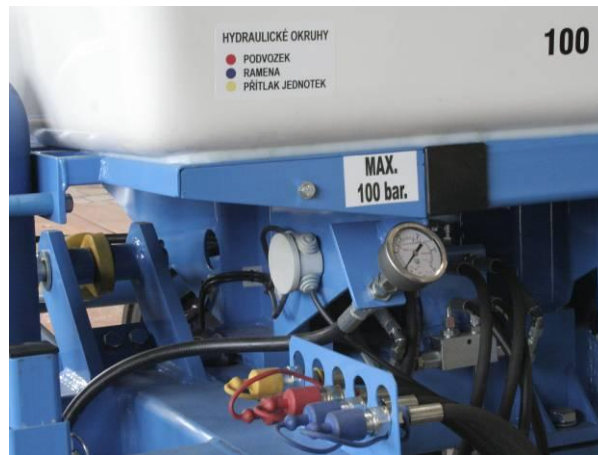
Fig. 7 Connecting Hydraulic Circuits
